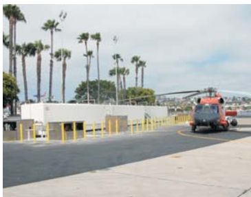
Jayhawk helicopter refueling at 75 GPM
